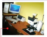
Light and fluorescence research microscope Leica DMRHC with Leica DC 3000f digital camera and data analysing system Image Pro Plus.
