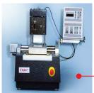
**Exact Grunding system** for cutting, embedding and grinding very hard tissues.
