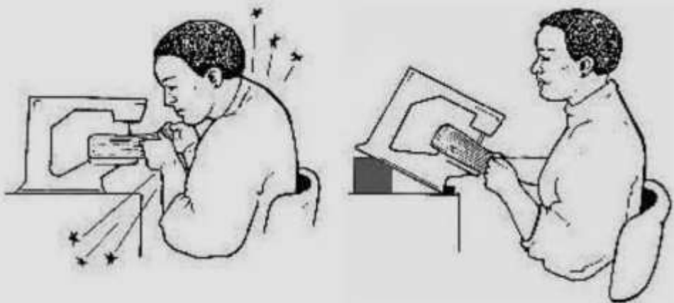
Bent neck (and wrists) improved by tilting the machine.
